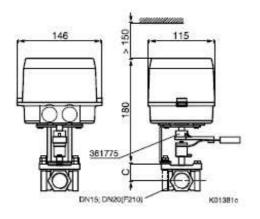
M3R three-way valve with ASM124 actuator
