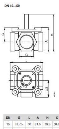
M3R three-way valve with AR30 actuator
