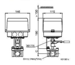
M4R four-way valve with ASM105/115 actuator
