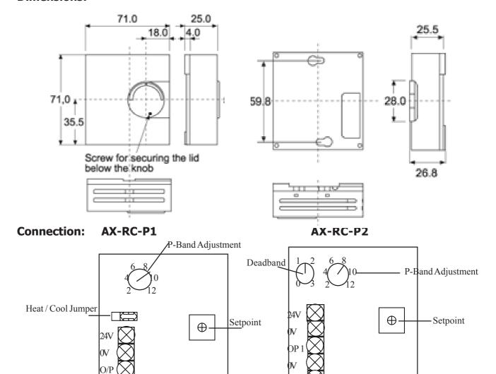
Output 1 = Heating Output 2 = Cooling
