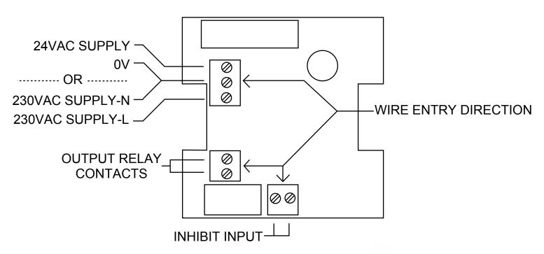
WARNING - The Inhibit input is indirectly connected to the 24VAC / 230VAC supply and can cause electric shock if touched
