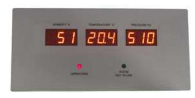
The Display unit is designed for fitting into an aperture in the wall, and will display the Temperature, Humidity and Differential pressure outside an Operaing Room or ICU. It will also give LED indication of when the room is in use. The unit accepts 3 x 0-10V and 2 Volt free signals from the BMS and is operated from 24Vac. The unit has a "Microban" label and the whole front plate clips to the top of the back box
