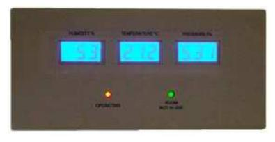
The Display unit is designed for fitting into an aperture in the wall, and will display the Temperature, Humidity and Differential pressure outside an Operaing Room or ICU. It will also give LED indication of when the room is in use. The unit accepts 3 x 0-10V and 2 Volt free signals from the BMS and is operated from 24Vac. The unit has a "Microban" label and the whole front plate clips to the top of the back box
