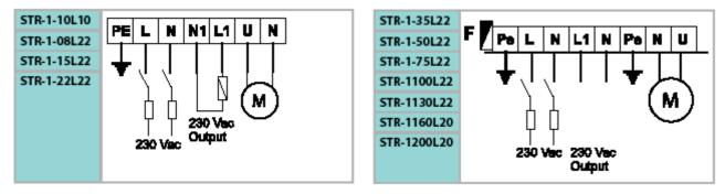
Type L22: by exchanging the fastonclip connectors on the transformer, one can adjust the order of switching and the voltage corresponding to each step of the switch.
