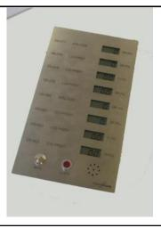
The Display unit is designed for fitting into an aperture in the wall, and will display Temperature, Humidity or Differential pressure or other Parameters- mounted on a brushed stainless steel plate. The unit accepts upto 8 x 0-10V from the BMS or Sensors and is operated from 24Vac. The whole front plate screws to the back box for ease of installation. The unit comes complete with a sounder , alarm LED and mute button
